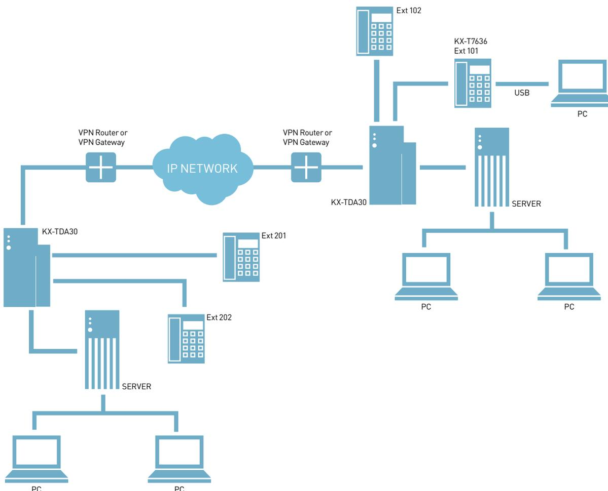
IP network infrastructure, which already exists in the majority of companies, can now carry voice along with data. Designed to support convergence through a modular structure, the system allows a harmonious migration towards VoIP, allowing voice and data communication to work within the same network.
